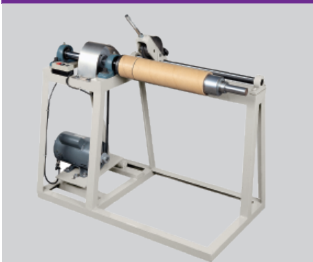
FPT-500 Manual type Cutting length: 20 - 450 mm
